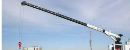
The 7543 is the newest addition to the Tiger Crane family and comes with the latest in crane innovations. Featuring 30.5 ft of all hydraulic reach in a lightweight package, the 7543 is the model for operators that require extended crane reach in a medium duty truck package.
