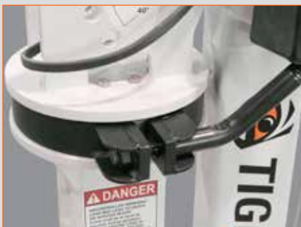
Slew bearing for easy rotation and manual band brake
